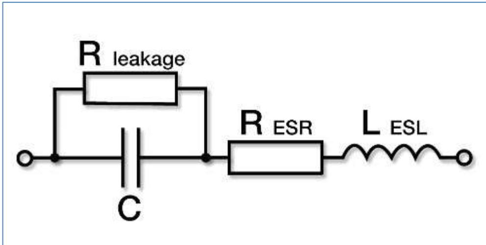
the real world, capacitors have other electrical properties than capacitance.
